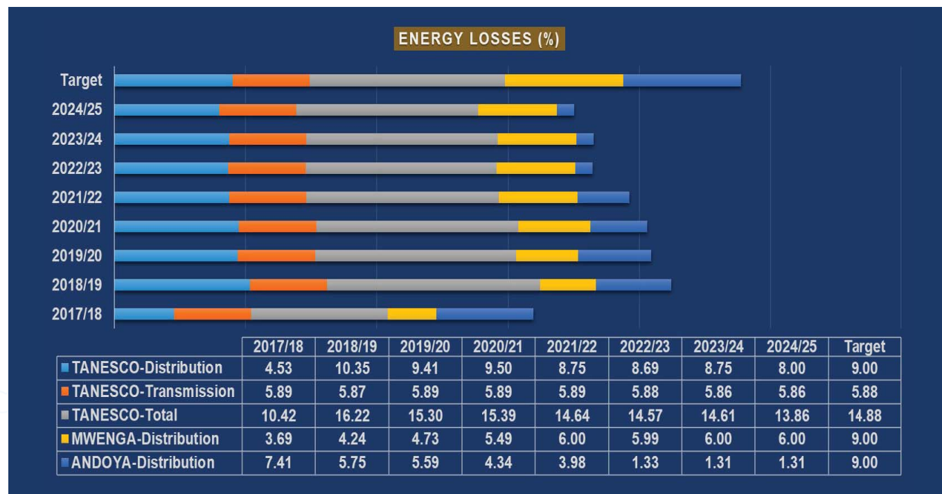
Figure 68: Energy Losses (FY 2019/20 – FY 2024/25)
