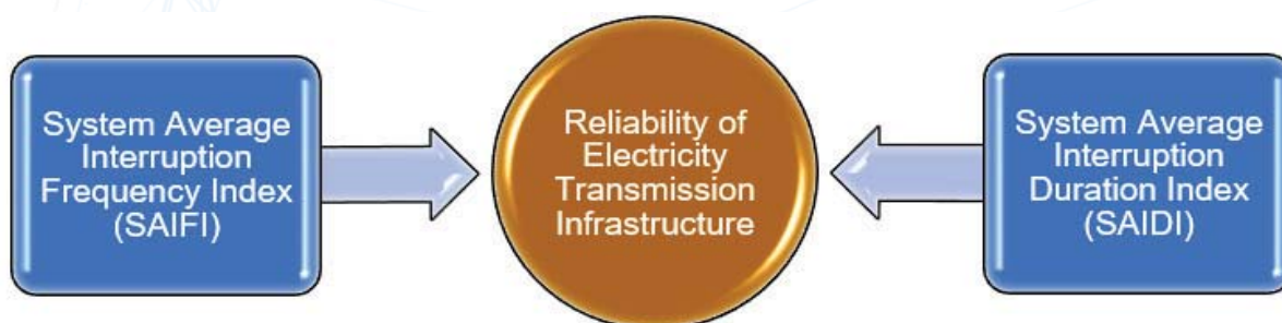
Figure 53: Description of Electricity Transmission Infrastructure Reliability Indices
